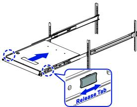
13 Secure the switch to the rack using the screws.
