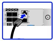
**2** Connect the other end of the Ethernet cable to a network. The Management port LED (Link/Activity LED) lights green when the network link is established.
