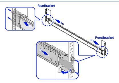
The switch supports front and rear rail installations.
