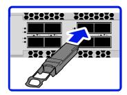
**3** Repeat the above procedures to install additional QSFPDD modules. For more information about the QSFPDD port LED behavior when the network link is established, refer to "LED Indicators of T9032-IX9".
