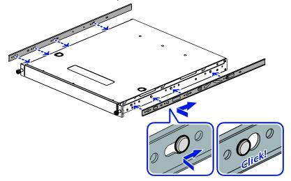
**8** Secure the inner rail to the switch with the screws.
