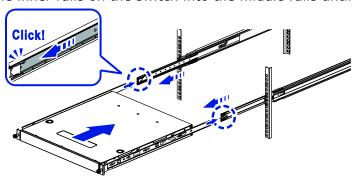
Pull/push the blue release tab on the inner rails and push the switch all the way to the rear of the rack.
